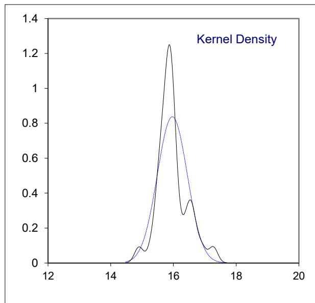
Determination of Density at 15°C on sample #21275; results in kg/m<sup>3</sup>
