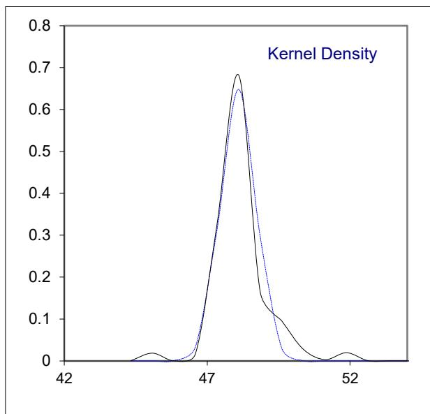
Determination of Kinematic Viscosity Stabinger at 50°C on sample #21275; results in mm<sup>2</sup>/s
